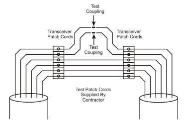
OTDR readings will be used to ensure proper installation and to troubleshoot faults. OTDR signature traces will be used for documentation and maintenance. An OTDR provides an indirect estimate of the loss of the cable plant; generally, more accurate or reliable values will be obtained by using an Optical Power Meter. For fibers that are identified in the plans to be left unterminated, an OTDR shall be used to test end-to-end attenuation.
