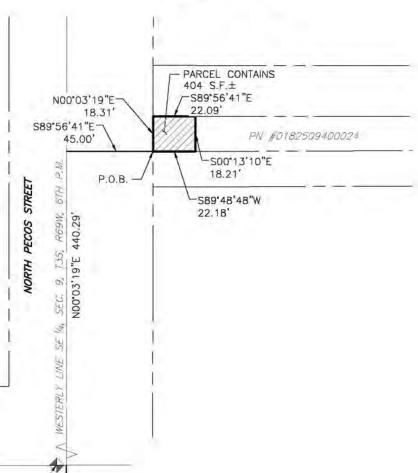
N/4 CORNER SEC. 16, T35, R68W, 6TH P.M. FOUND 2-1/2" ALUM CAP IN RANGE BOX PLS #37601 5' W.C. POINT OF COMMENCEMENT
