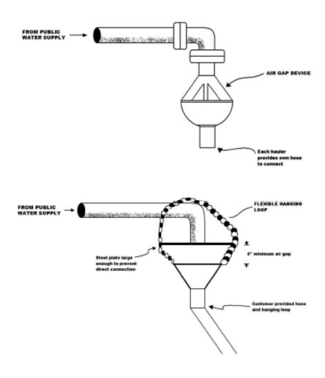
Figure 8.1 Acceptable water loading stations
