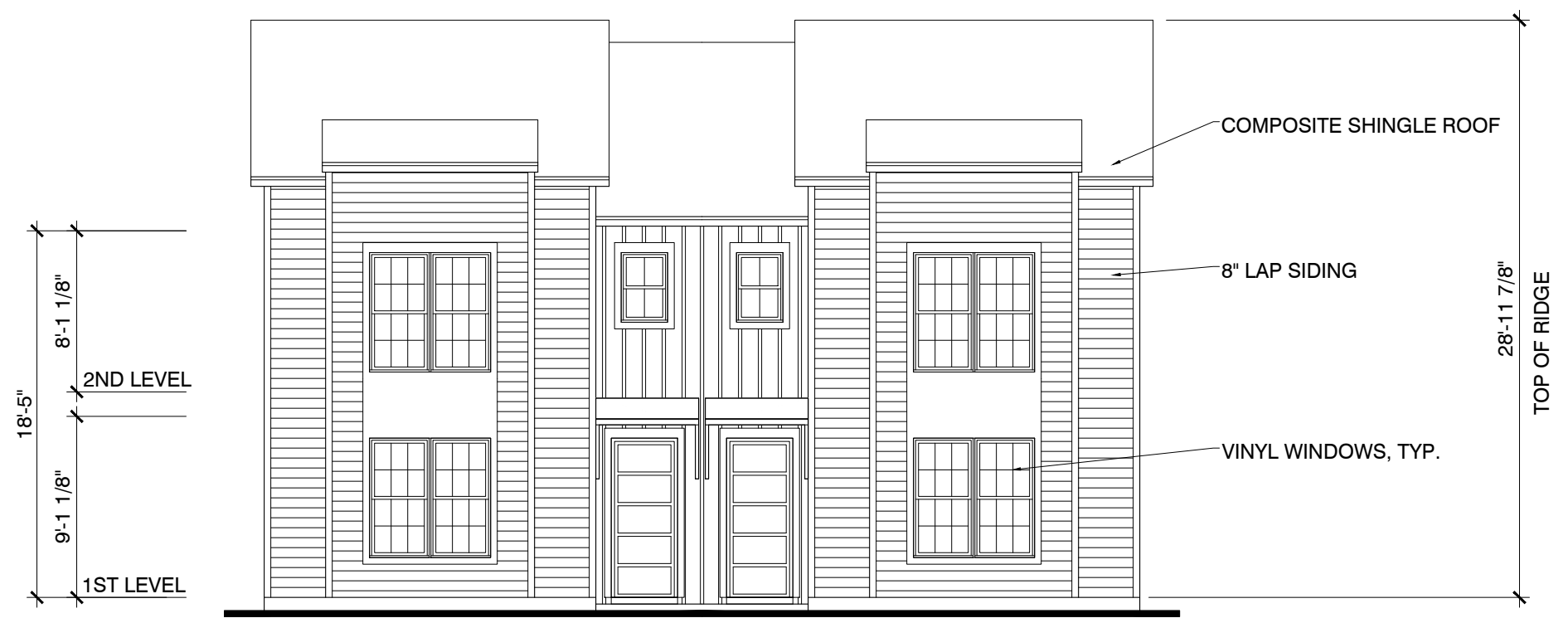
2 UNIT BUILDING - FRONT ELEVATION SCALE: 1/8"=1'-0"
