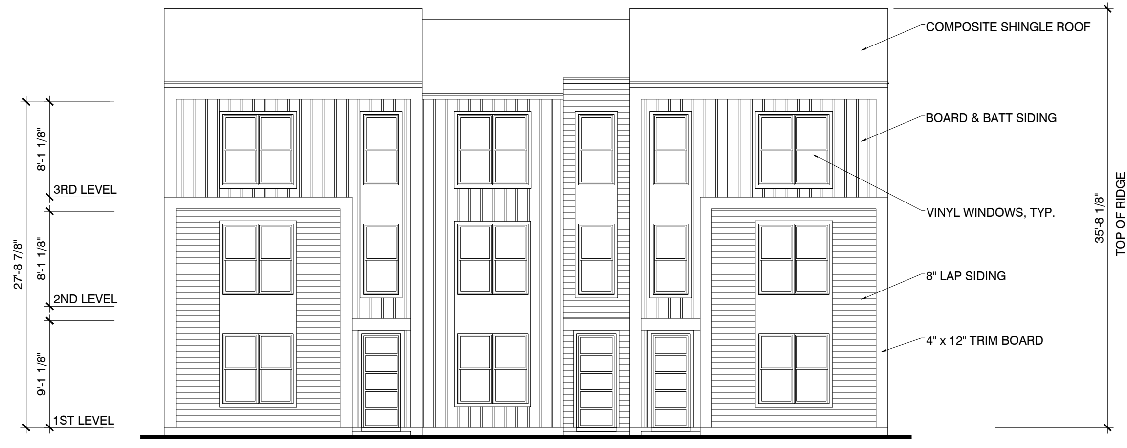
3 UNIT BUILDING - FRONT ELEVATION SCALE: 1/8"=1'-0"
