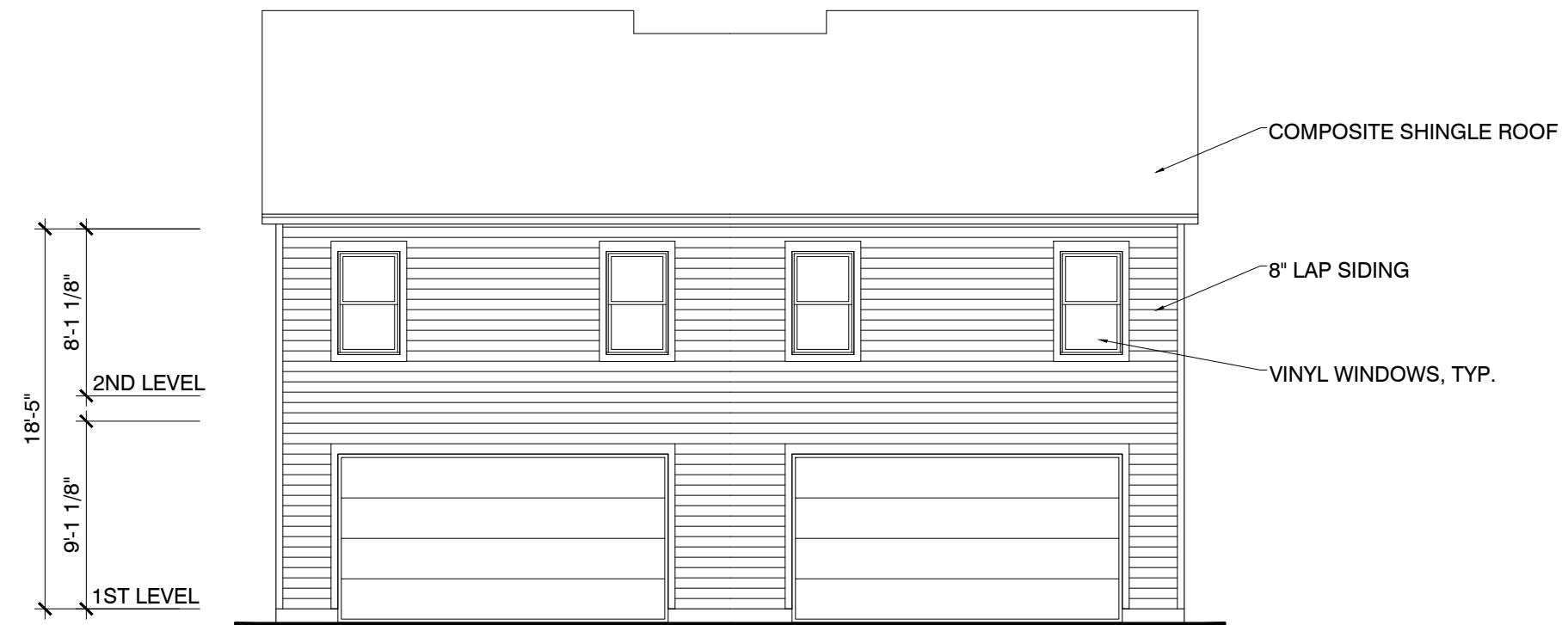
2 UNIT BUILDING - REAR ELEVATION SCALE: 1/8"=1'-0"
