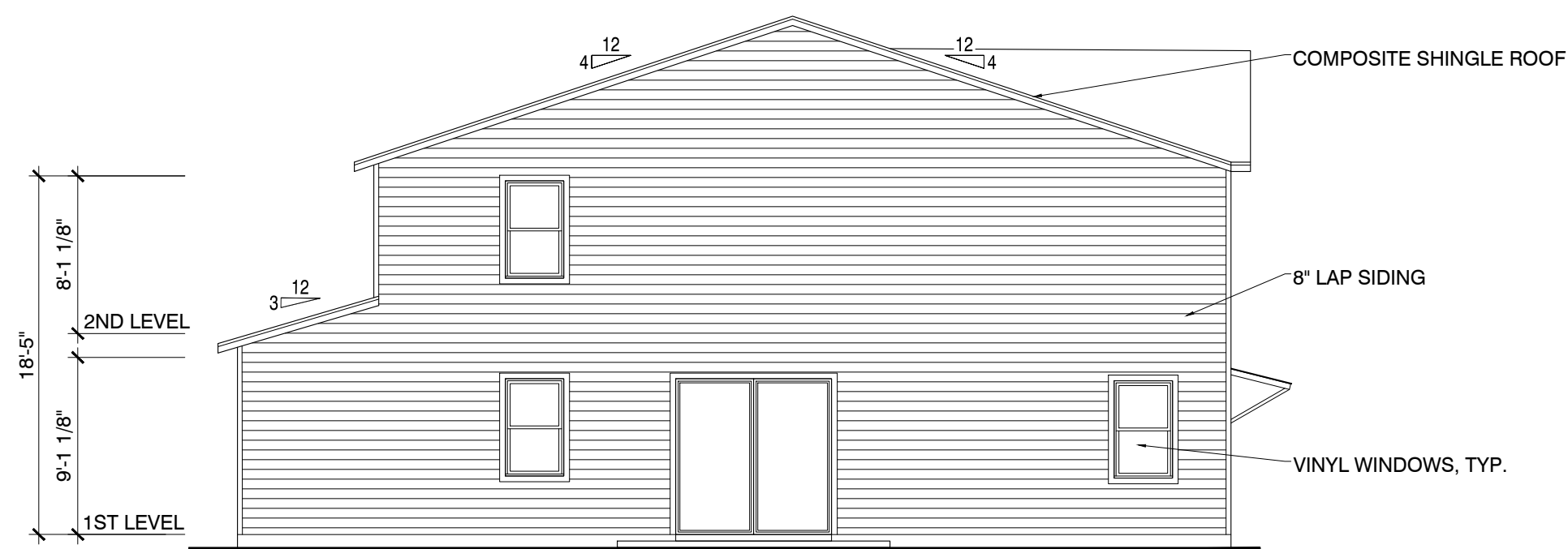
2 UNIT BUILDING - LEFT SIDE ELEVATION SCALE: 1/8"=1'-0"
