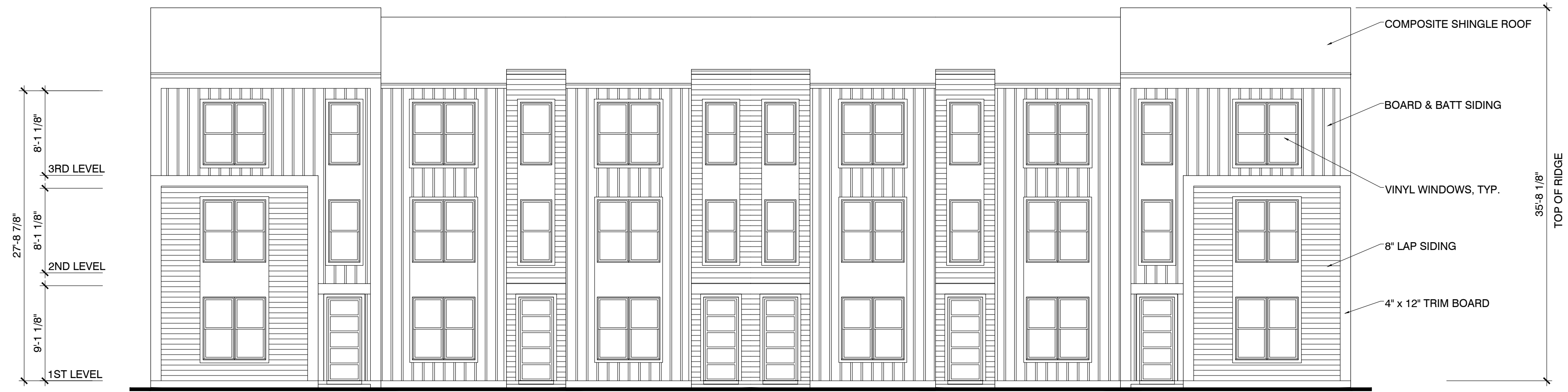
6 UNIT BUILDING - FRONT ELEVATION SCALE: 1/8"=1'-0"
