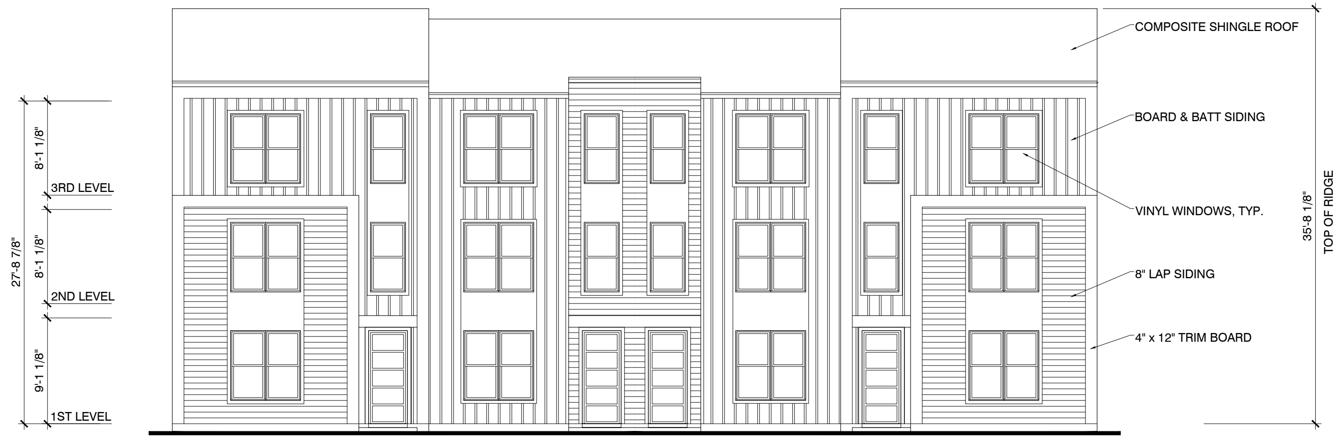
4 UNIT BUILDING - FRONT ELEVATION SCALE: 1/8"=1'-0"
