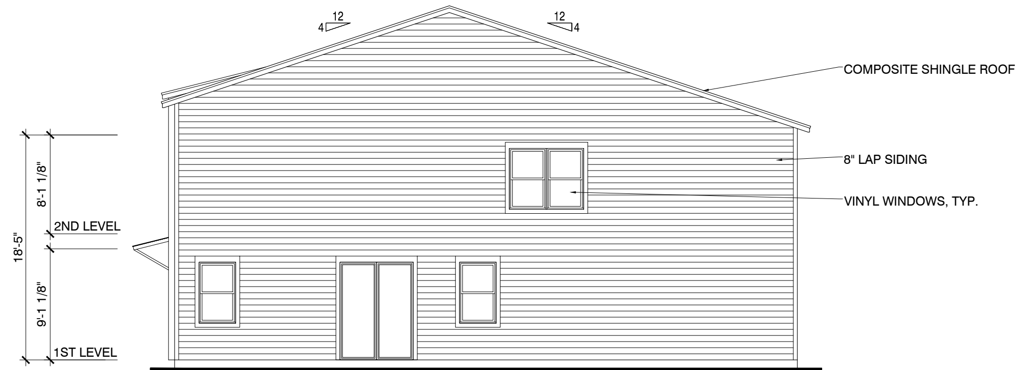
2 UNIT BUILDING - RIGHT SIDE ELEVATION SCALE: 1/8"=1'-0"
