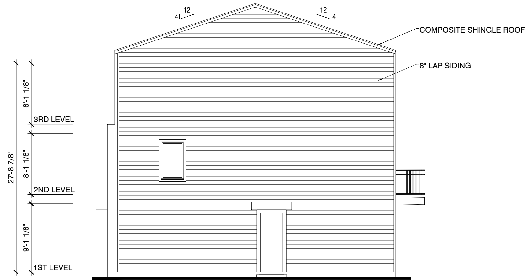
4 UNIT BUILDING - RIGHT SIDE ELEVATION SCALE: 1/8"=1'-0"
