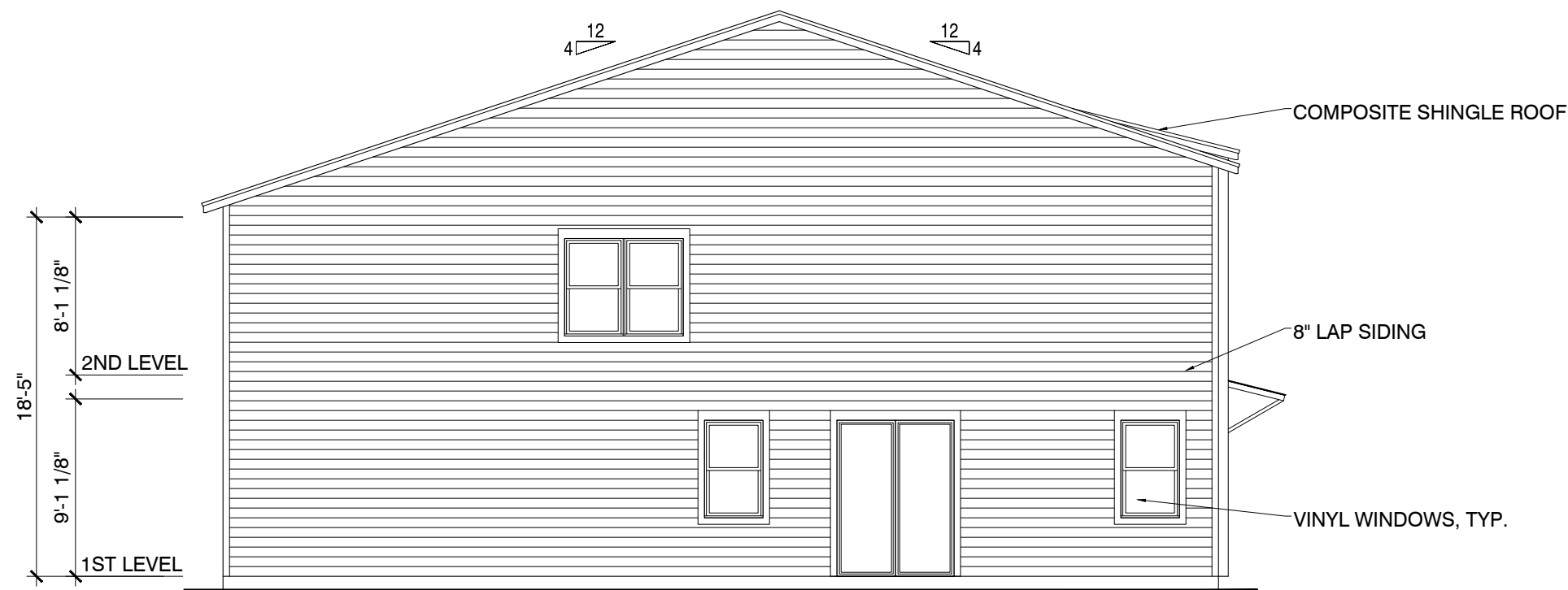
2 UNIT BUILDING - LEFT SIDE ELEVATION SCALE: 1/8"=1'-0"
