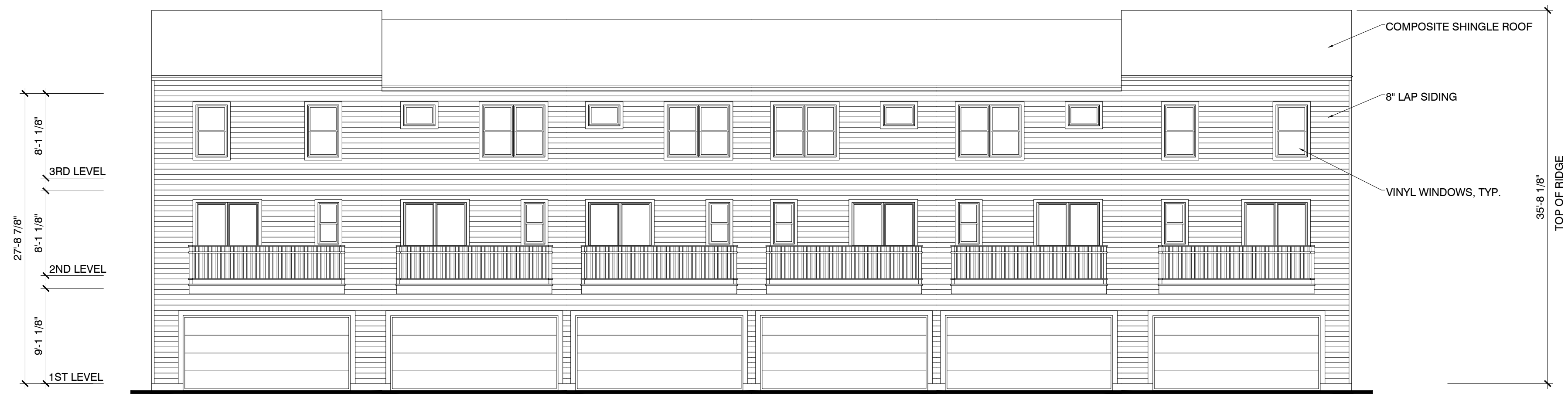
6 UNIT BUILDING - REAR ELEVATION SCALE: 1/8"=1'-0"
