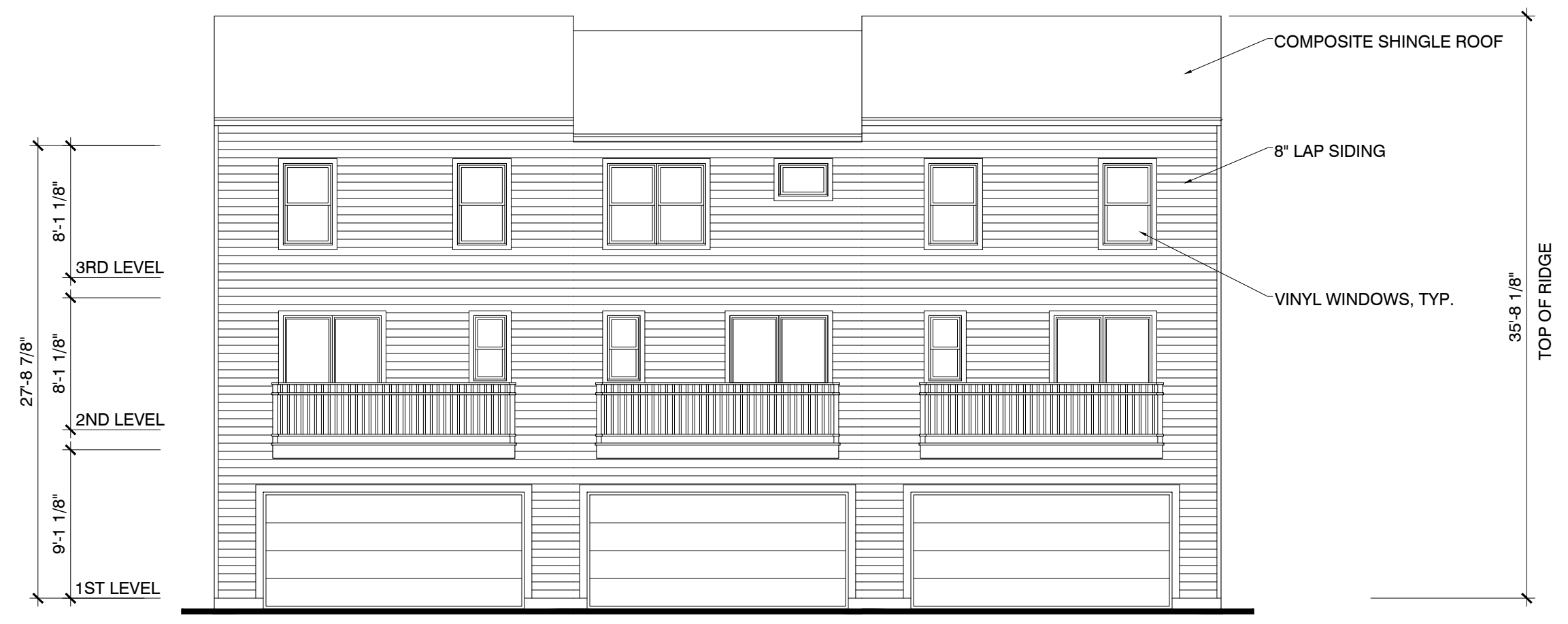
3 UNIT BUILDING - REAR ELEVATION SCALE: 1/8"=1'-0"
