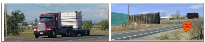
Figure 6. Typical sand truck and traffic control signage for well pad. Trucks slowing down to turn is one of the primary concerns, and the "Trucks Turning" sign alerts drivers to the change in traffic pattern.
