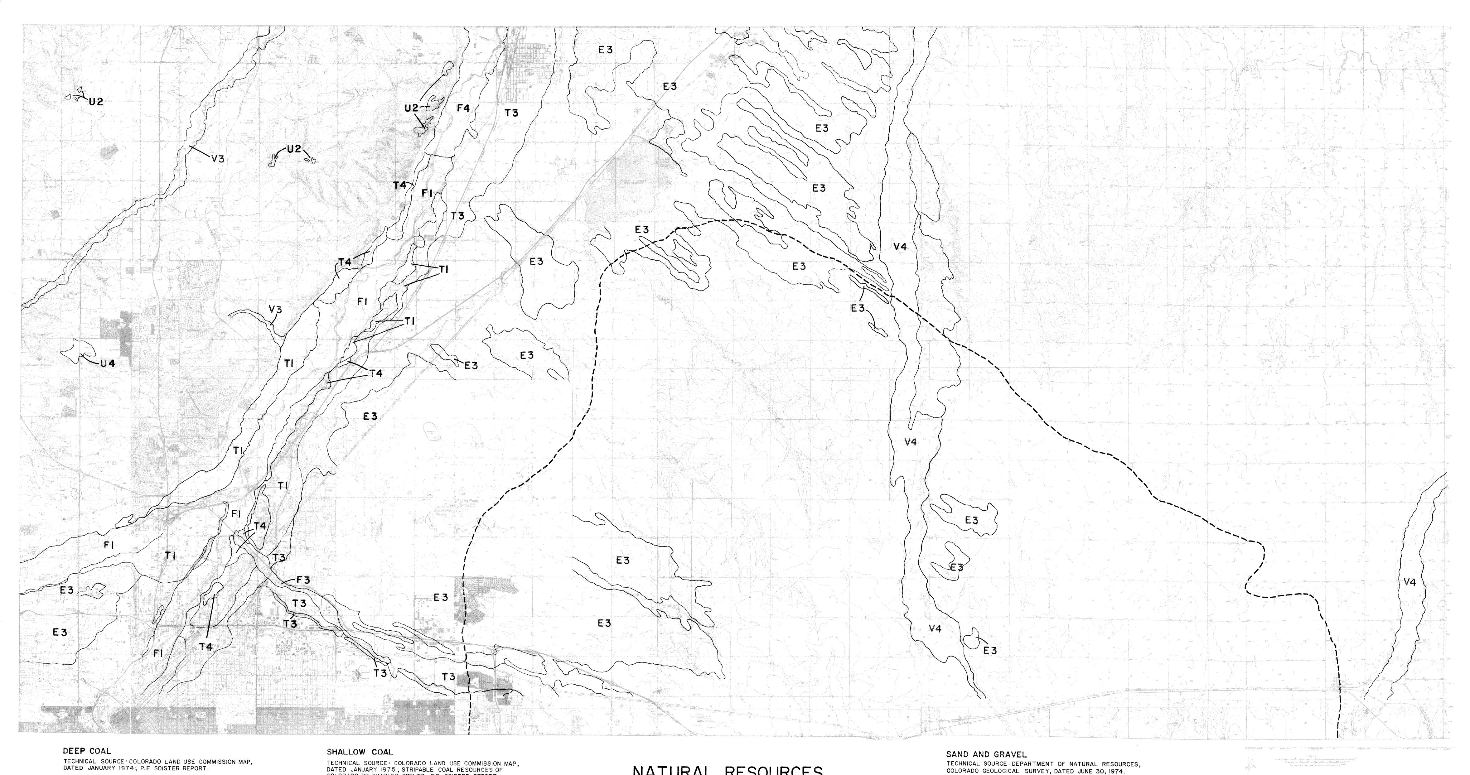
HIGHER GRADE SUB-BITUMINOUS COAL DEPOSITS EXIST FROM 500' TO 1600' BELOW THE SURFACE IN CONJUNCTION WITH THE LARAMIE FORMATION FOR THE WESTERN 3/4 OF ADAMS COUNTY AND CONTINUES ON THIS MAP. THE EXTENT AND QUALITY IS UNKNOWN. EXTRACTION, HOWEVER, WOULD HAVE TO BE THROUGH SHAFT MINING, AND IS CONSIDERED UNLIKELY IN THE FORSEEABLE FUTURE. TECHNICAL SOURCE: COLORADO LAND USE COMMISSION MAP, DATED JANUARY 1975; STRIPABLE COAL RESOURCES OF COLORADO BY CHARLES SPELTZ; P.E. SOISTER REPORT.
