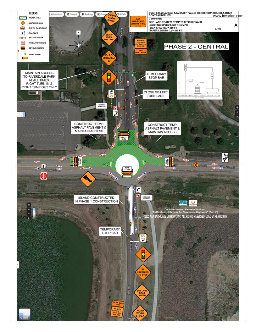
www.invarion.com LEGEND CONSTRUCT TEMP. ASPHALT PAVEMENT & MAINTAIN ACCESS - WORK AREA CONSTRUCT TEMP. ASPHALT PAVEMENT & MAINTAIN ACCESS - TYPE 3 BARRICADE - FLAGGER - TRAFFIC DRUM TEMPORARY STOP BAR Henderson Rd Menderson Rd Henderson Rd 💝 Henderson Rd PHASE 2 - EAST ISLAND CONSTRUCTED IN PHASE 1 CONSTRUCTION Date: 1.28.22 Author: AAA STAFF Project: HENDERSON ROUND-A-BOUT CONTRACTOR: ESI ONE LANE ROAD W/ TEMP TRAFFIC SIGNALS:
