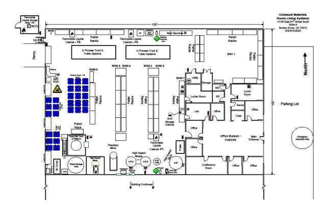
The above diagram is an example only. Your facility floor plan may be depicted much differently than the above. Critical information that should be included in all facility site plan diagrams are chemical inventory locations/storages, shut-off switches/valves/processes, loading docks where chemicals are received/shipped, and any designated safe areas.
